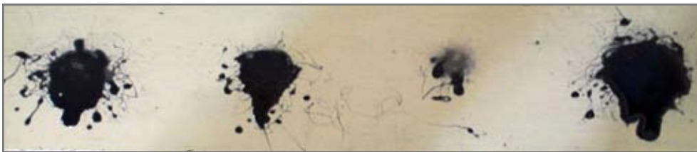
Spray pattern using a commercial grade lubricant.
